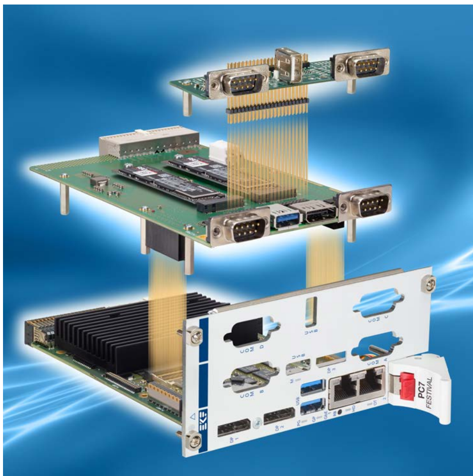
12HP Assembly w. PCZ-NVM & C32-FIO
